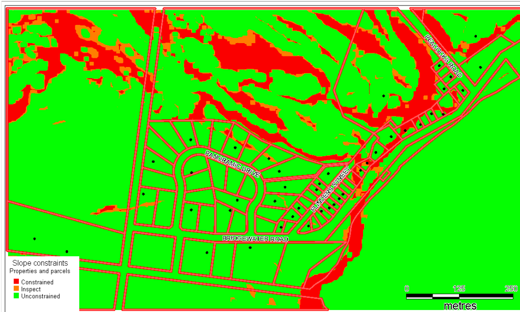
Map 6: Slope constraints in Cape Bridgewater in relation to properties and parcels. The Code prohibits the consideration of land for wastewater absorption fields if it has steep slopes, or is within 3 metres of an adjacent allotment for pressurised trench systems (red buffer), or 1.5 metres of an adjacent allotment for irrigation systems (pink buffer). Here slopes are shown in three classes – 0-18% as being unconstrained, 19-21% as requiring inspection and >21% and as being constrained. Dots represent dwelling locations. A 60m buffer from the foreshore was not mapped because it would not have adversely impacted any developments.
