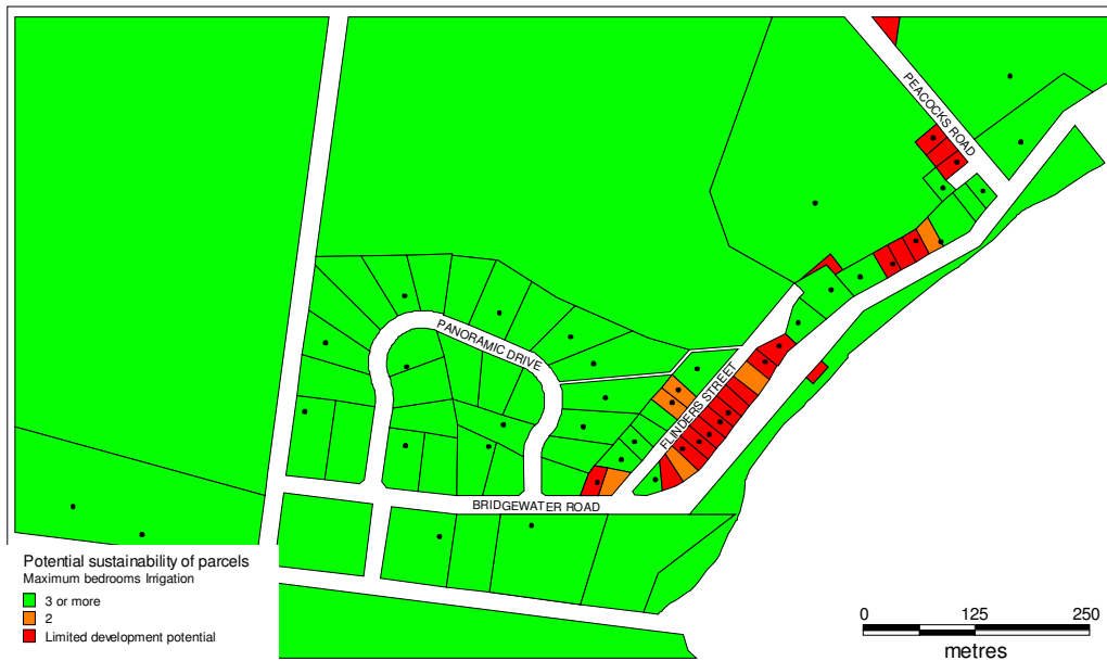
Map 10: Potential sustainability for parcels using irrigation systems. It takes into account the absorption field recommendations in for AS/NZS category 1 soils in table 3, an allowance of 450m 2 for impervious surfaces and constraints in map 6. Compared to map 9, there are a number of additional parcels that would be unable to deal with wastewaters onsite. Dots represent dwelling locations.
