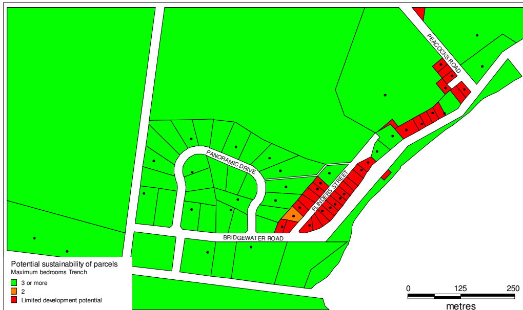
Map 8: Potential sustainability for parcels using trench systems on AS/NZS category 1 soils. It takes into account the absorption field recommendations for AS/NZS category 1 soils in table 6 of the report introduction, an allowance of 450m 2 for impervious surfaces, and the constraints shown in map 6. The map incorporates a reserve field and assumes that each dwelling would use an all-waste system and a dosing pump. This is map of onsite system sustainability should each parcel be developed and indicates that severe problems might emerge in the foreshore area if Cape Bridgewater was to be fully developed using traditional trench technologies. Dots represent dwelling locations.
