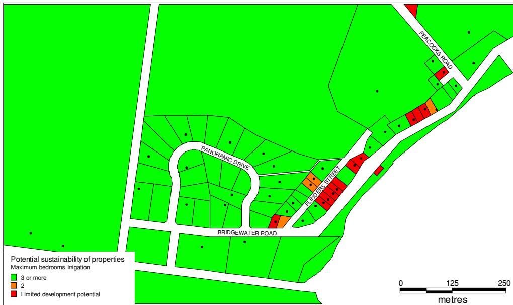
Map 9: Potential sustainability for properties using irrigation systems. It takes into account the absorption field recommendations for AS/NZS category 1 soils in table 3, an allowance of 450m 2 for impervious surfaces, and the constraints shown in map 6. If upgraded to irrigation systems, there are properties that would remain unable to deal with wastewaters onsite, and nearly all of these are already developed. Dots represent dwelling locations.
