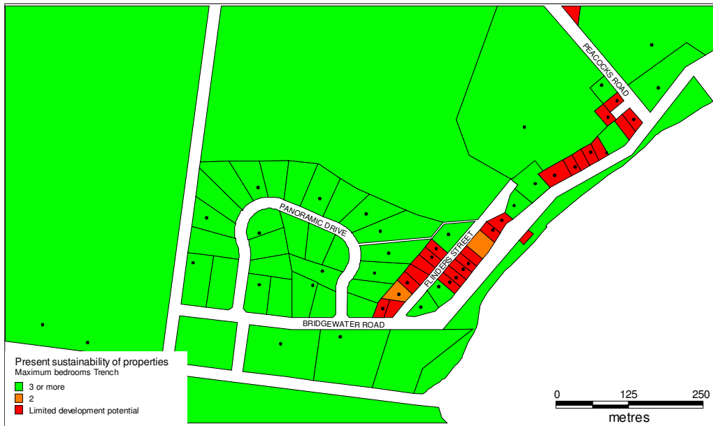
Map 7: Present sustainability for properties using trench systems. The map incorporates a reserve field and assumes that each dwelling would use an all-waste system and a dosing pump. It takes into account the absorption field recommendations for AS/NZS category 1 soils in table 6 of the report introduction, an allowance of 450m 2 for impervious surfaces, and the constraints shown in map 6. Many properties along the foreshore are too small to accommodate a trench system and a reserve field, and clusters of developed properties with limited development potential suggest that there are probably already wastewater problems in the town. 4
