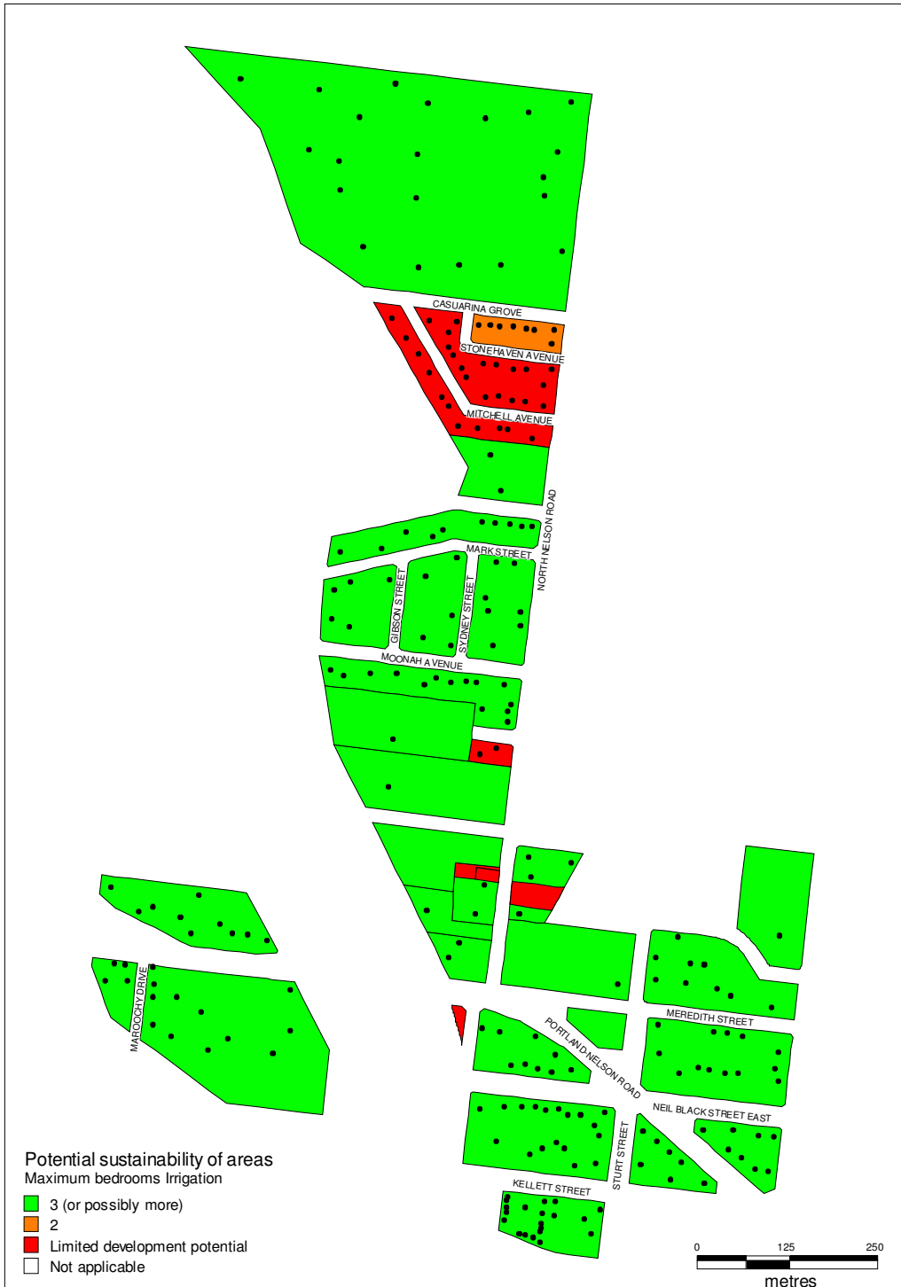
Map 5: Potential sustainability of irrigation systems in areas within a fully developed Nelson. It takes into account the absorption field recommendations for AS/NZS category 1 soils in table 3, an allowance of 450m 2 for impervious surfaces, and ignores the constraints shown in Map 6. Most of Nelson would benefit from a change to irrigation technology over time. However the area surrounding Mitchell Avenue and south of Casuarina Grove remains a concern. It is near-fully developed and the many of the blocks are around 500m 2 .
