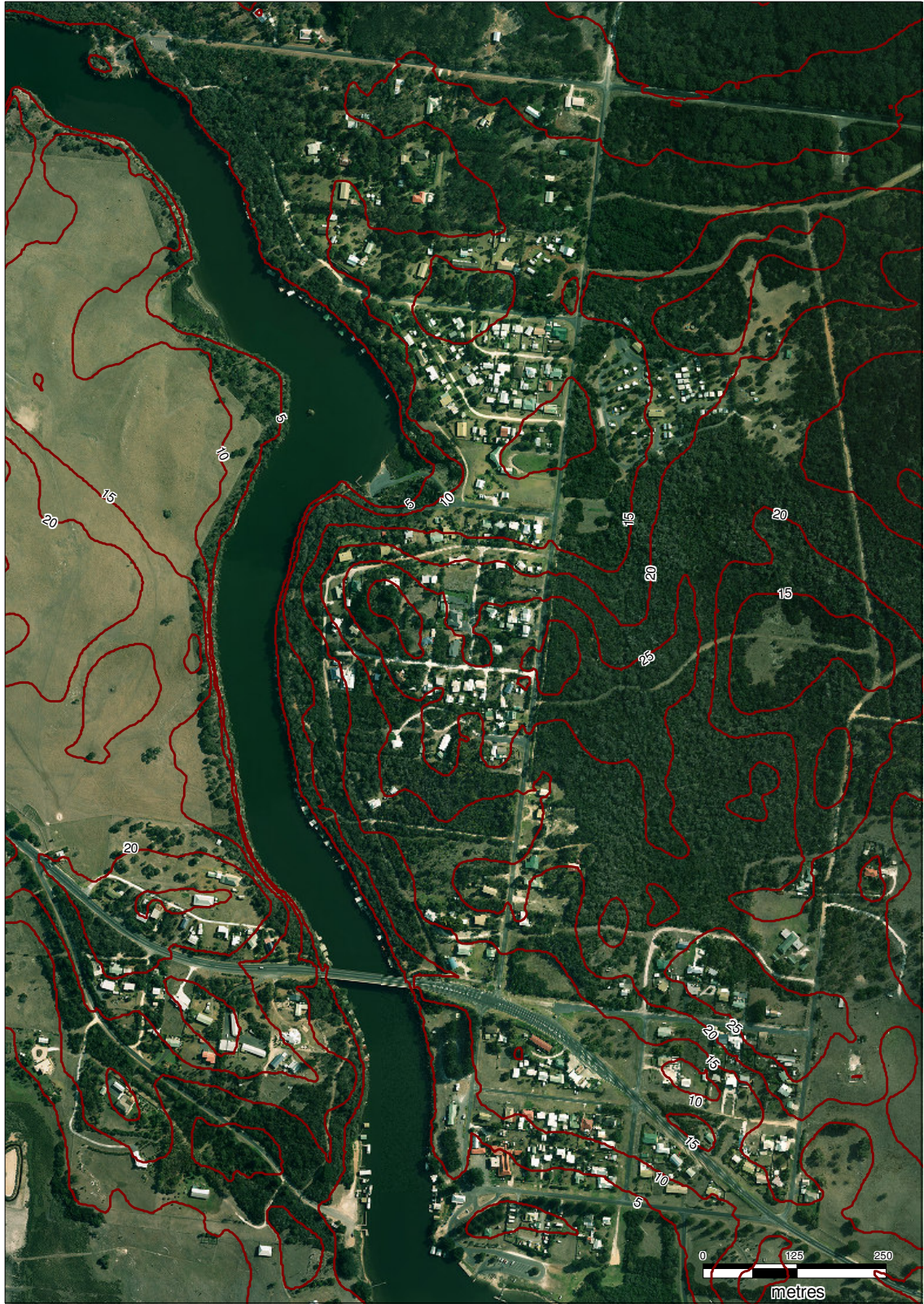
Map 1: Air photo of Nelson overlaid with 5m contours. Although there is less relief to the north, Nelson is uniformly an AS/NZS category 1 soil.
