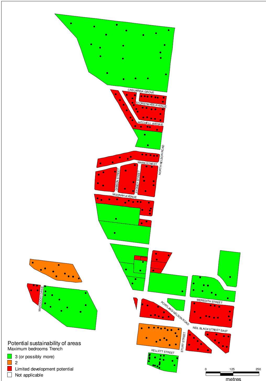
Map 4: Potential sustainability if Nelson were to be fully developed using trench technology. The map assumes that each parcel has a dwelling using an all-waste system and a dosing pump. It does not consider the constraints shown in Map 6. It takes into account the absorption field recommendations for AS/NZS category 1 soils in table 6 of the report introduction, and an allowance of 450m 2 for impervious surfaces. Some areas that are sustainable at present would not be if fully developed using trench systems. The area in Kellett Street has changed status because the map does not reflect non-domestic wastewater circumstances.
