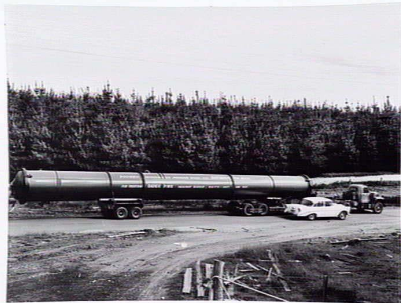
Figure 55: Dartmoor Pine Mill trucks carrying Boliden impregnation Pressure Vessel Source: Lyle Fowler (1891-1969) State Library of Victoria Accession No IAN01/07/89/22
