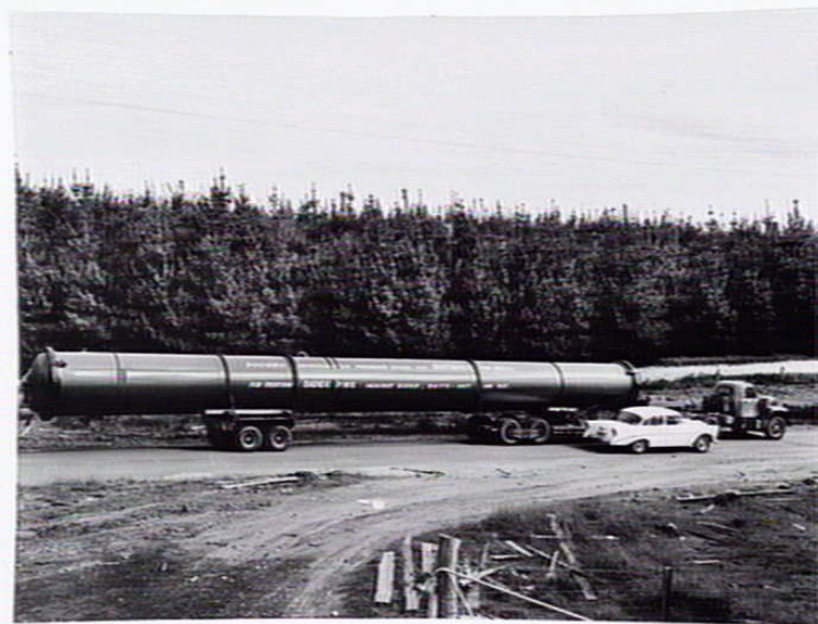
Figure 60 Dartmoor pine mill trucks carrying Boliden impregnation Pressure Vessel Lyle Fowler (1891-1969) State Library of Victoria Accession No IAN01/07/89/22
