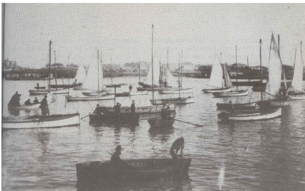
Portland fishing fleet c1892. The evolution of the 'couta boat up till this time can be traced in this one photo. There are boats of barely 18 feet in length, there are a number of about 20 feet, and there are one or two carved boats which could be up to 26 feet long. Freeboard on most of the boats is low, which made them easier to row, and all boats are rigged with a standing lugsail. Larger vessels in the background are sailing lighters and fishing boats.
