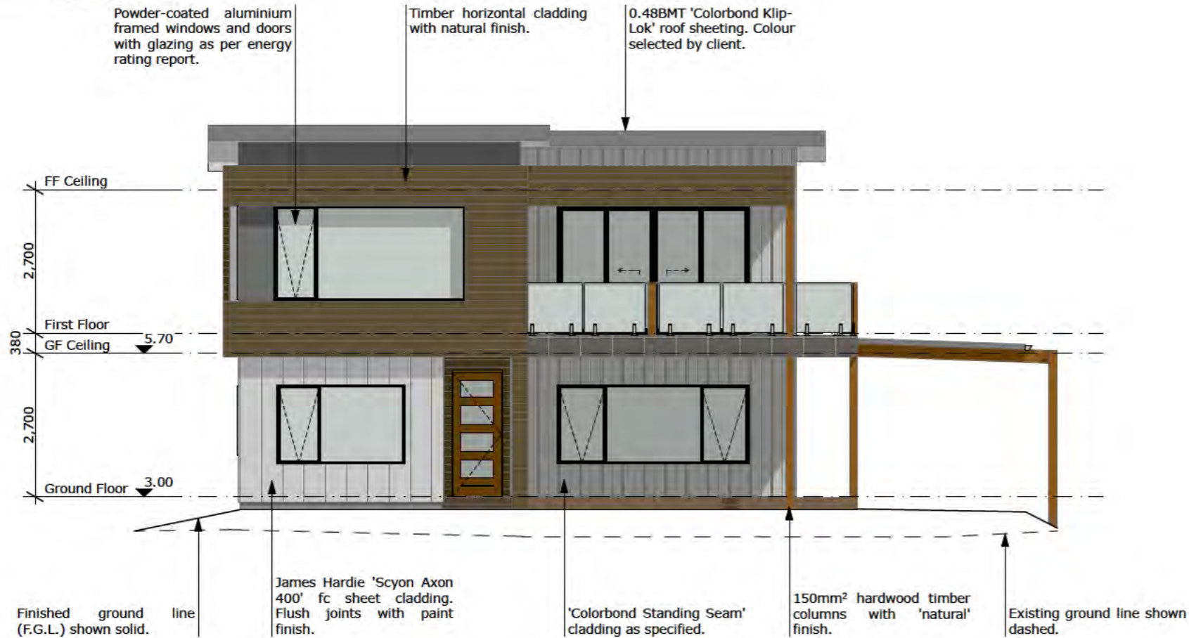
2 Elevation Proposed East SCALE: 1:100
