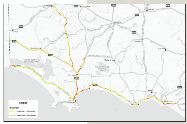
Figure 9: Resurfacing and rehabilitation treatments required under predicted conditions (by 2024), VicRoads
