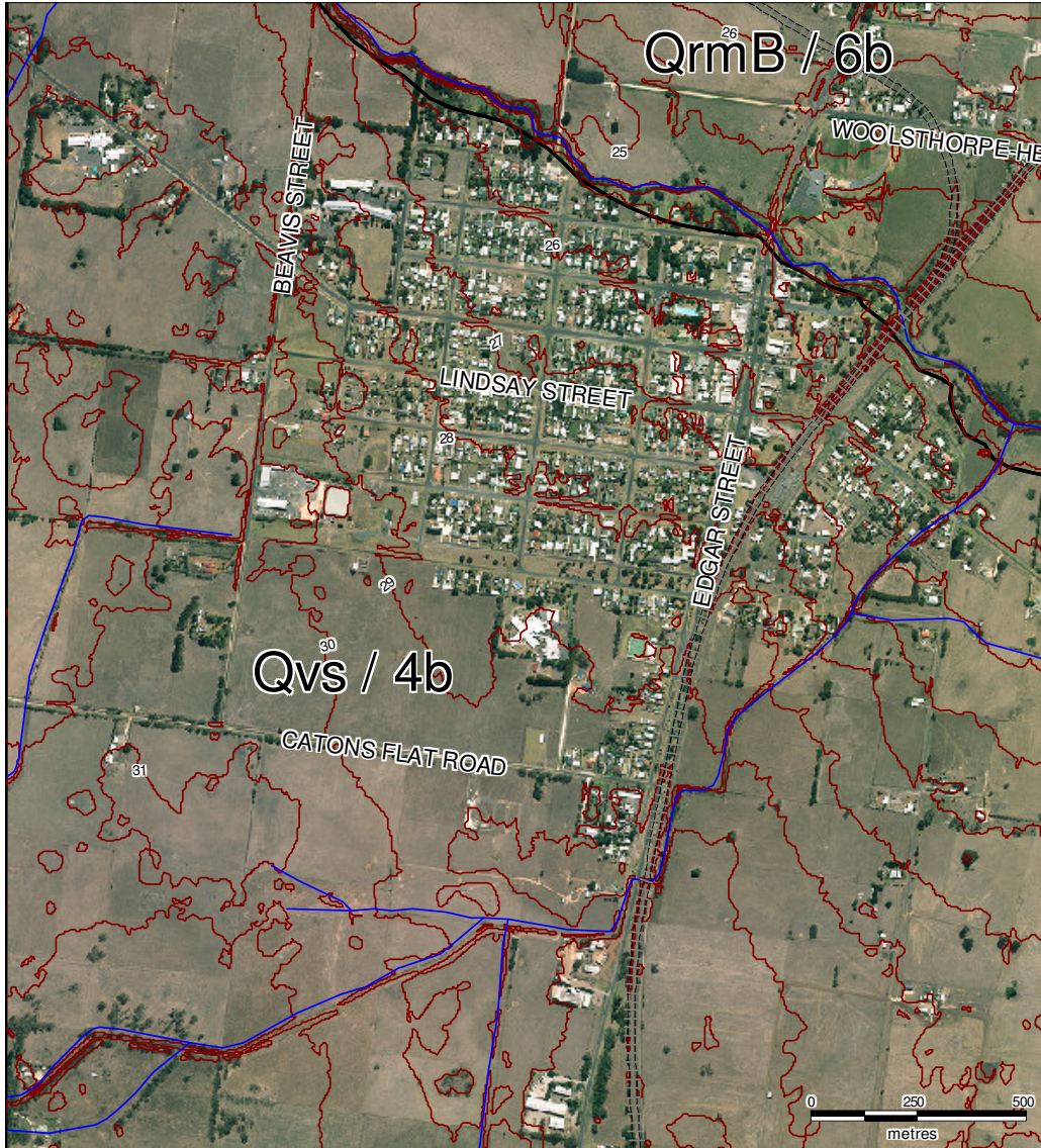
Map 1: Air photo of Heywood overlaid with 1m contours. Soils are based on QrmB and Qvs geology (AS/NZS category 6b and 4b soils, respectively). Unsewered blocks are crosshatched.
