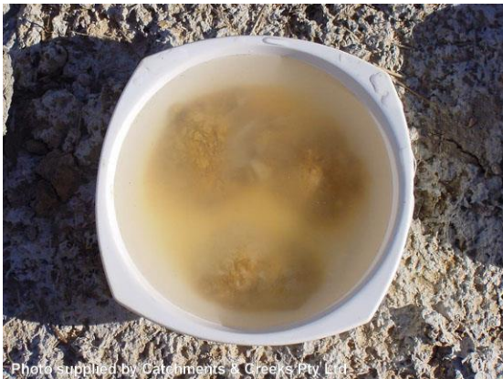
Field testing a dispersive soil
